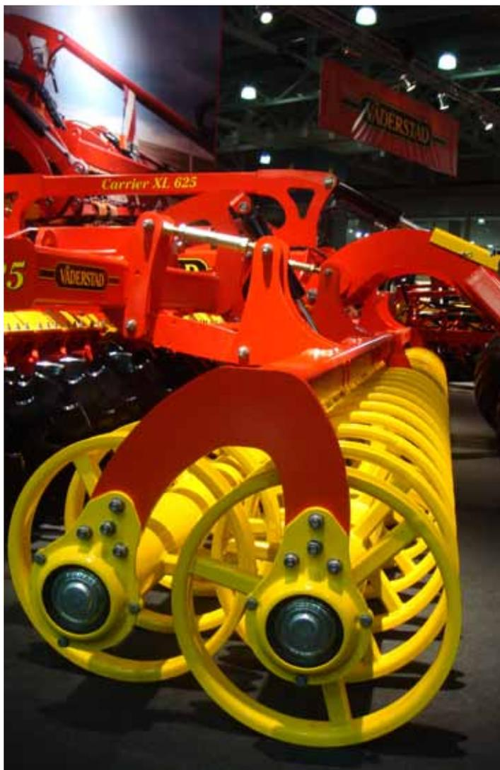
The essential novelty in the Carrier design is the increased disc diameter: L – 51 cm, XL – 61 cm (45 cm on previous models). This change eases work on fields with a large amount of crop residue, including crude types, such as maize and sunflower stubble.
