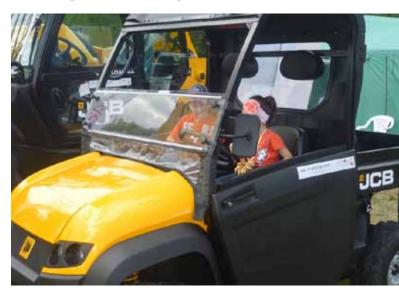
JCB WORKMAX, caused quite a stir. Both adults and children sought to test drive it. These trucks are fitted with Yanmar three-cylinder diesel engines, 14.9 kW. Weighing a mere 710 kg, they provide a total lifting capacity of 600 kg.
