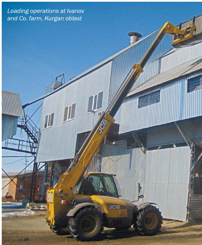
structure distributes the stress over the entire jib length, thus reducing fatigue and preventing likely breakage in the nose part.
