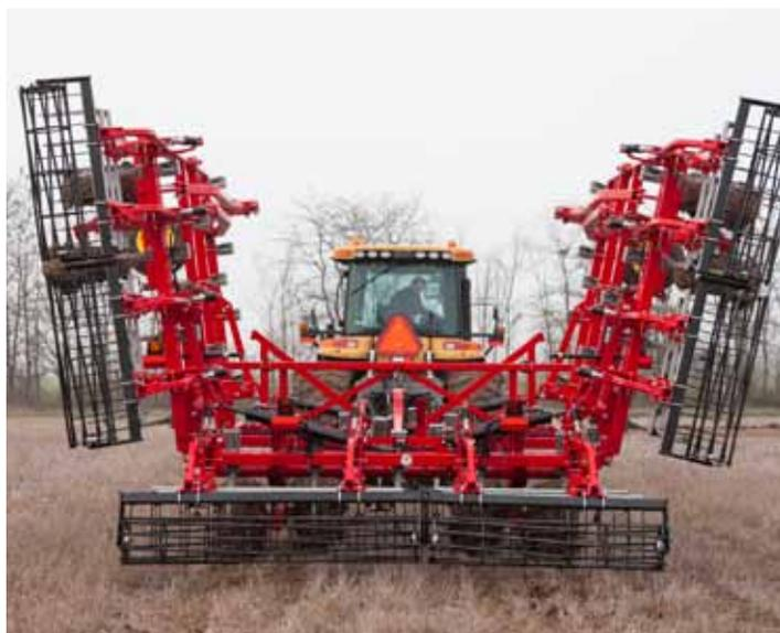
hp tractors. Extra strength is provided by a sixth beam added to the rear of the main frame. The floating suspension mechanism helps the machine to closely follow the profile of the field being treated, all of which ensures superior cultivating quality.
