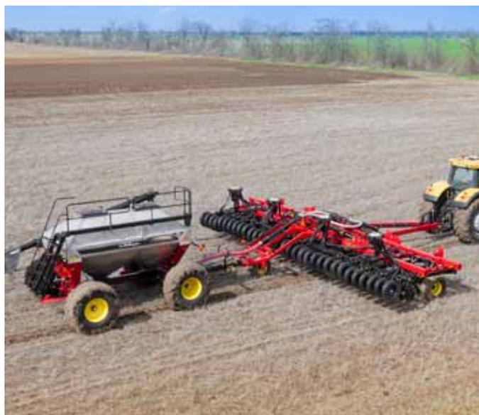
is the use of a patented technology of single-disc coulters positioned opposite
