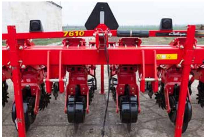
Challenger 7600 cultivators are designed for strip tilling. When using this technique, the soil is tilled only in the strip into which the seeds are introduced. Thus, the between-the-row space remains untouched. Stilling is used for growing tilled crops. The Challenger 7600 series of cultivators includes
