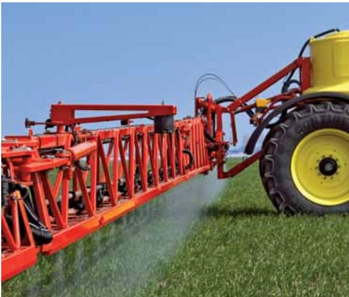
The triangular beam profile specifically developed for this model assures maximum reliability and fully protects the nozzles, hoses and pipelines. Offered as an option are pumps with an output of 200, 250, 400, 500 l/min.
