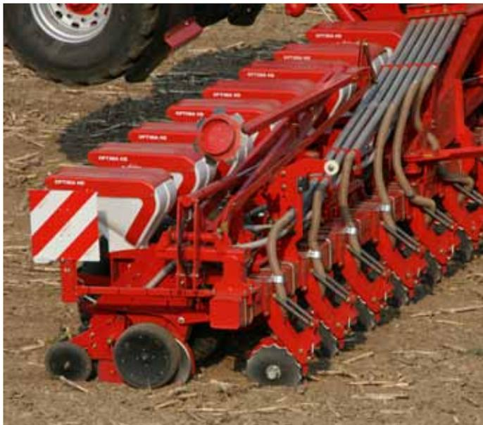
The new precision drill is ideally suited for large farms. The operating width of 12 m (16 rows and the inter-row spacing of 70 mm) plus the 4,000-litre fertiliser bin enable the TF seeder to work 100 hectares per day! This reduces the unit costs of using the tractor and its operator.
