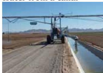
A canal is dug in the centre across the field. The system moves over the edge with a lowered pump which picks up water from the canal. This system is suited for small fields, since it enables towing and turning around for greater area coverage. The flexible suction hose ensures minimum investment because it is suitable practically for every workable canal in the earth.
