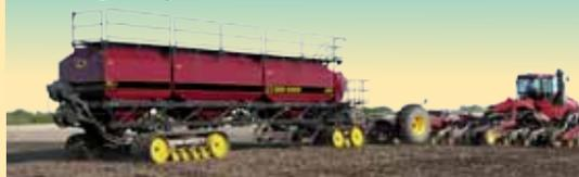
The hopper is divided into four variously sized sections for storing seeds and fertilisers: 10,500, 16,800, 16,800 and 1,400 litres. Filling takes up just 15 minutes since the seeds and fertilisers are delivered simultaneously.
