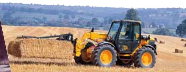
Despite its compactness, the loader features the operational capabilities of the well known JCB multi-role telescopic loaders with a side-mounted engine. The gear pump hydraulics system ensures the output of up to 126 l/min. The
